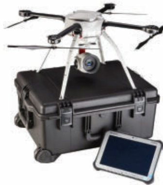
A SkyRanger unmanned aerial vehicle system complete with an HDZoom30 payload and flight control tablet.
