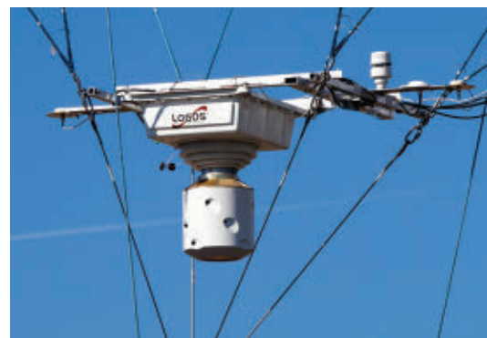
Logos Technologies’ Simera wide-area motion imaging sensor can monitor city-sized areas.
